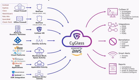
CyGlass collects NetFlow, Syslog, VPC, and other logs via a data collector layer which ingests data, parses it into relevant formats, and transmits it to our Cloud AI engine via a secure SSH channel.
